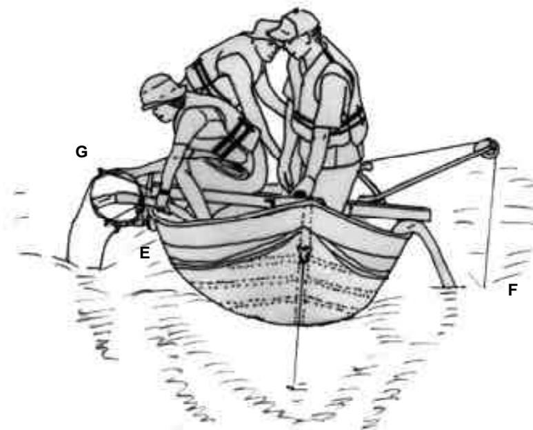
Figure 3: Collection procedure: (E) turn on the pump and the water comes out from the hose; (F) low the sampler with the winch and (G) put the collecting net in position.
