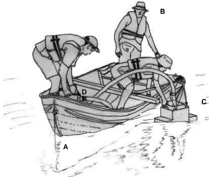
Figure 2: Collection procedure: (A) put the anchors and ballasts in the river; (B) the boat worker maintains the boat motor in operation; (C) put the sampler in the water and (D) fill the pump and the hose with water.
