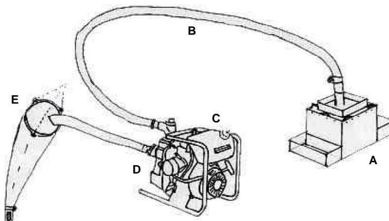
Figure 4: Disposition of the equipment parts in operation: (A) entrance of the material in the Suction sampler; (B) passage of the material through the hose; (C) passage of the material through the pump; (D) exit of the material from the hose and (E) collection of the material in the net.
