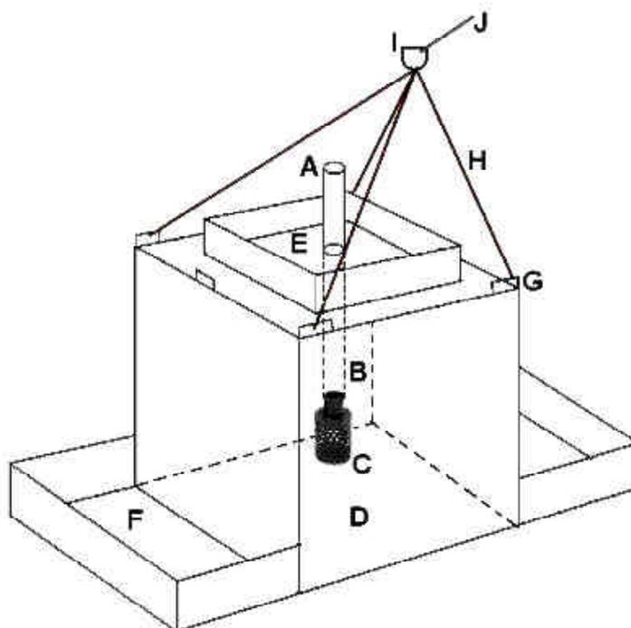
Figure 1: Three-dimensional view of the Suction sampler: (A and B) extremities of the tube; (C) filter; (D) lower part of the box; (E and F) ballasts installation places; (G) handle; (H) strings; (I) clamp and (J) steel cable.
