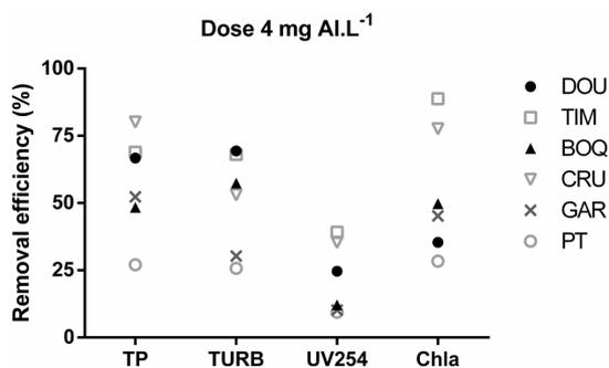
**Figure 2.** Removal efficiency (%) for total phosphorus (TP), turbidity (TURB), humic substances (UV<sub>254</sub>) and chlorophyll-a (Chl-a) in raw water from Dourados (DOU), Timbaúba (TIM), Boqueirão (BOQ), Cruzeta (CRU), Gargalheiras (GAR) and Passagem das Traíras (PT) reservoirs, after coagulation-flocculation with the dose of 4 mg Al L<sup>-1</sup> and 30 minutes of sedimentation.
