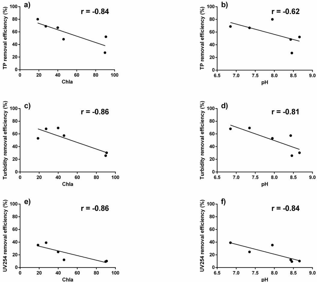
**Figure 3.** Correlations between chlorophyll-*a* concentration and pH with total phosphorus (TP), turbidity and UV<sub>254</sub> removal efficiency (%) based on the dose of 4 mg Al L<sup>-1</sup>.
